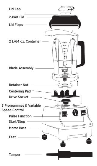
**Tamper:** The tamper allows you to accelerate the process of very thick and/or frozen mixtures that cannot be processed in a standard blender. Using the tamper maintains circulation by preventing air pockets from forming during blending.
